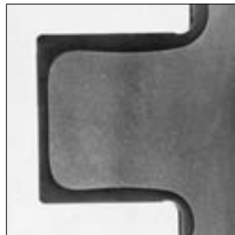
Figure 10: Raceways of a nose ring in a three-row roller bearing slewing ring
